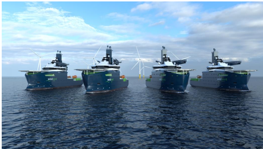
VARD 4 19 | CSOVs for Windward Offshore | Length of 87.5 meters | Accommodation for 120 POB
