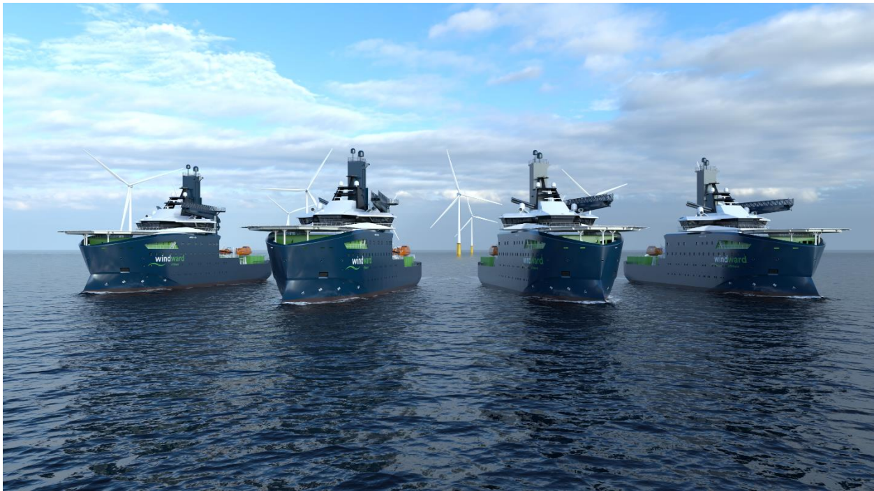
VARD 4 19 | CSOVs for Windward Offshore | Length of 87.5 meters | Accommodation for 120 POB
